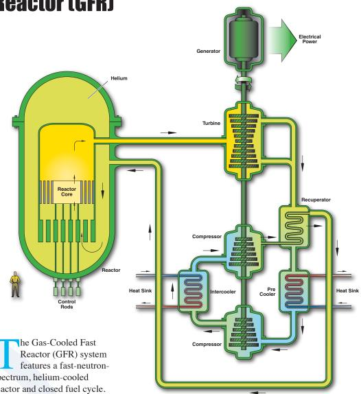
Through the combination of a fast spectrum and full recycle of actinides, the GFR minimizes the production of long-lived radioactive waste.
